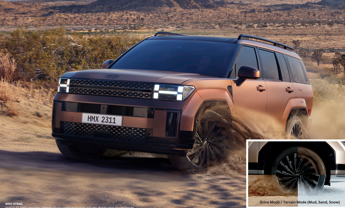
4WD HTRAC SANTA FE AWD provides optimal driving performance by actively distributing driving forces to the front and rear wheels depending on the situation.
